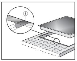
Grout lines (1) and the hatched area underneath the cooktop frame must be smooth and even. If they are not, the cooktop will not sit flush with the worktop and the sealing strip underneath the cooktop will not provide a good seal between the cooktop and the worktop.
